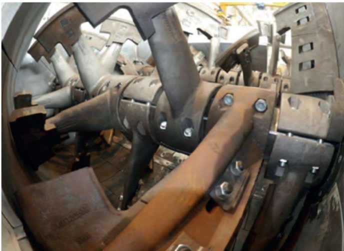
Mixing Blades inside Twin Shaft batching plant
