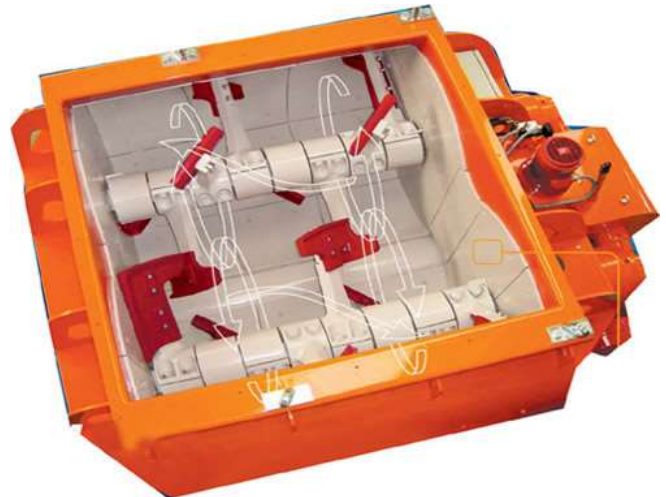
Counter Direction Movement of the blades
